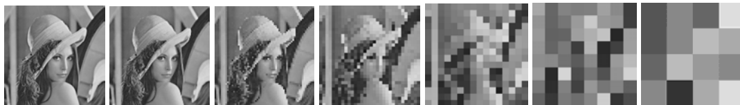
The Lena image with 256 by 256, 128 by 128, 64 by 64, 32 by 32, 16 by 16, 8 by 8, and 4 by 4 pixels
