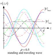
It is very convenient in practice to measure the rms value of a voltage. The rms value of a signal, which mathematically involves the time integration of the signal, is not a function of time. The rms value of a signal as a function of z is considered a standing wave even though it is not a function of time. This standing wave pattern is evident in the following plot.
