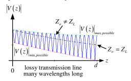
Although the VSWR might be mostly conveniently measured at the input of the line, the VSWR at the load can be significantly greater for a lossy line.
