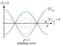
For other conditions, however, the two traveling waves do not appear to generate either a pure traveling or standing wave but a kind of combination of the two. An example of this situation follows. In this case, the minimum phasor amplitude,  $|V|_{min}$ , is not zero.
