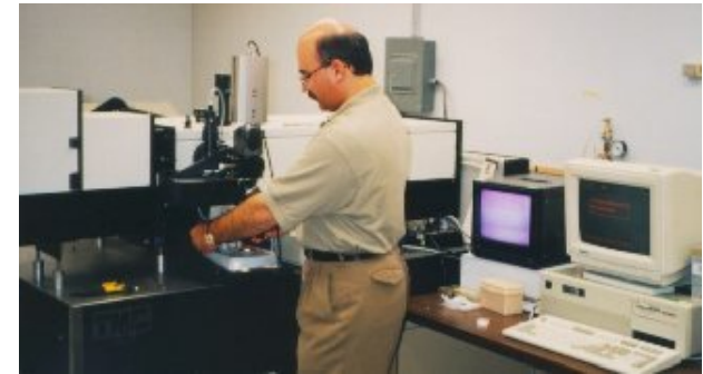
Dr. Bahram Roushani uses Raman spectroscopy to analyze the properties of thin layers (only a few atoms thick) of various materials with industrial and technological applications.
